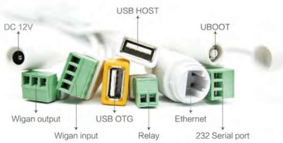
Connect with doors, gates, peripheral devices & network
